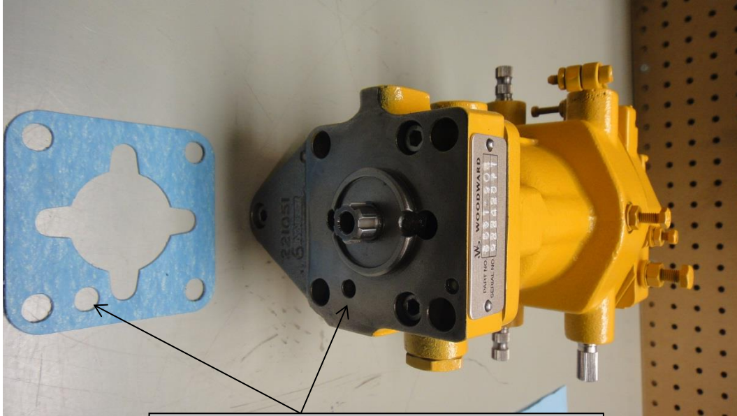
Caterpillar OIL SUPPLY inlet on base of Governor
